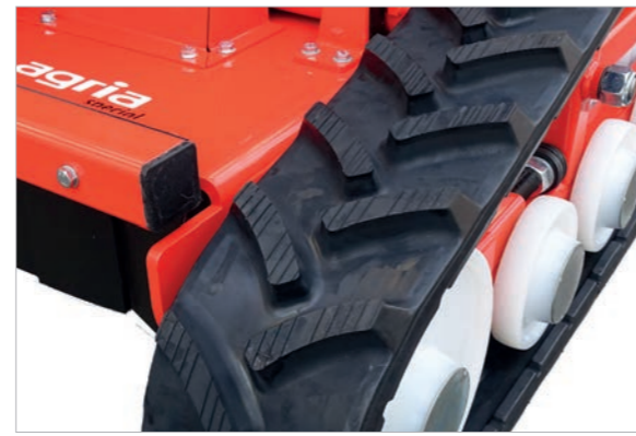
Crawler tracks with non-slip cleat-profile Ref. 9620 011
